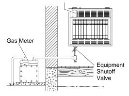
Figure 15 - Checking Gas Joints
